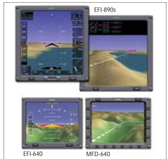
Universal Avionics is completing its FAA certification of a synthetic vision system that shows an egocentric view on the primary flight display and an exocentric view on the navigation display. The unit does not include highway-in-the-sky guidance.
